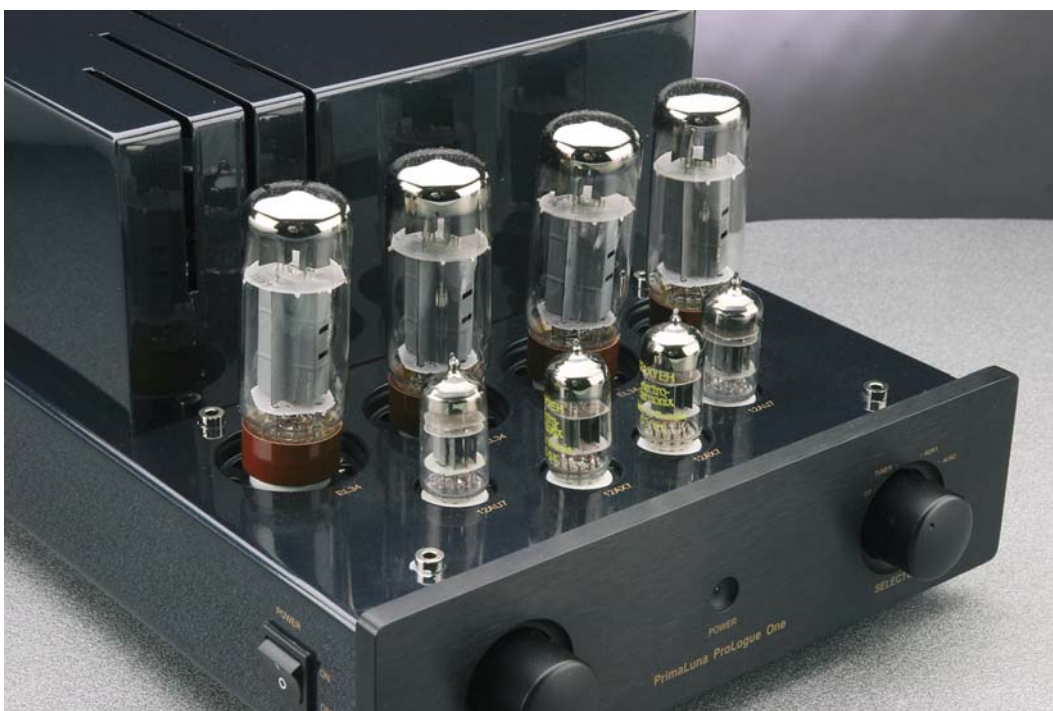
Power-amp section implements EL34 tubes which provides sufficient power in most applications. They are foregone by a pair of 12AX7 and a pair of 12AU7.
